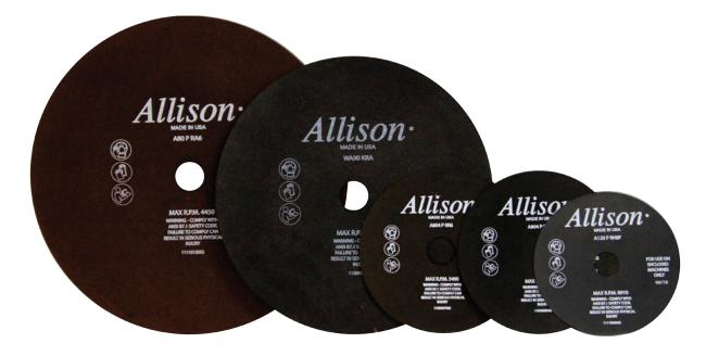
The cutting of electrical contact disc from tungsten rod is **Producers of Dental Alloys to cut:** commonly done wet with rubber bonded wheels 6 or 7 inches in diameter and from .013 to .017 inches thick, held to thickness tolerance of plus or minus one-thousandth of an inch. Similar wheels are used for accurate cutting of very small rod and tube sections and for cutting thin slots in various materials.
